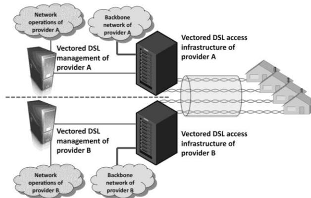
Figure 6 – Vectored DSL access infrastructure and management separately owned by multiple providers.
