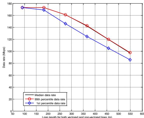
Figure 3 - Rate-reach plot for a group of 24 vectored lines when 24 non-vectored lines are also present in the same cable and their data rates are capped at 25 Mbps. For simulation details, see the Appendix.
