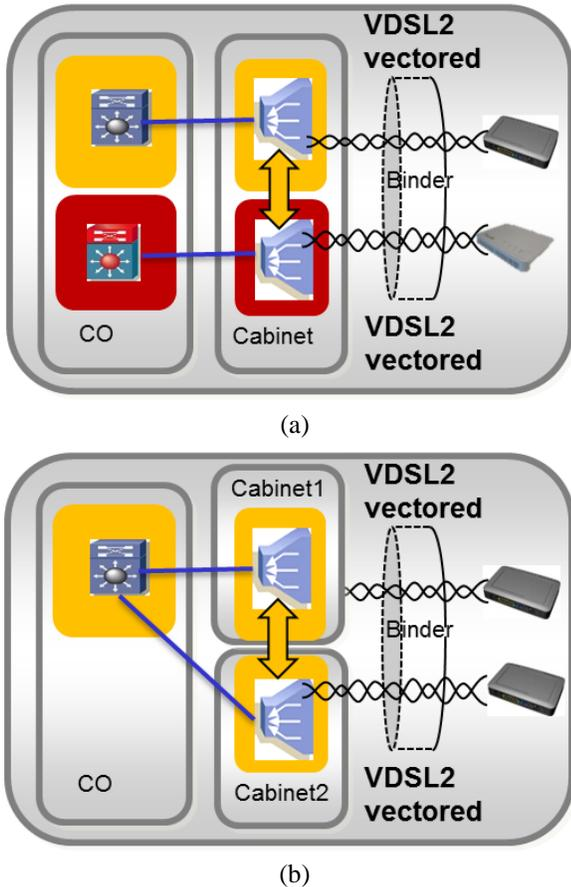
Figure 2 – An example of two DSLAMs connected via xDLV to create a larger vector group. The DSLAMs are owned by either (a) two different operators sharing the same cabinet area or (b) by the same operator.
