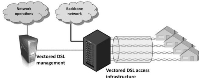
Figure 5 – Vectored DSL access infrastructure and management owned by a single provider.
