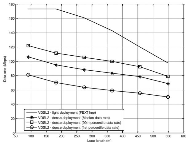
Figure 1 - Rate-reach plot for a group of 48 non-vectored VDSL2 lines for the two cases of light and dense (48% cable fill) deployment. For simulation details, see the Appendix.
