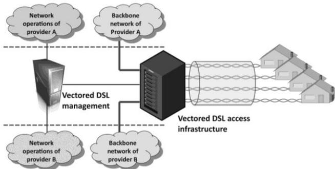
Figure 7 – Vectored DSL access infrastructure and management shared by multiple SPs. The DSLAM icon may represent a single DSLAM or also multiple ones (e.g., one or more DSLAMs per SP) and the DSLAMs of the various SPs can be cross-vectorized via xDLV.
